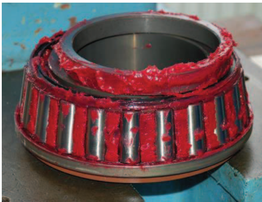
Fig. 2.1: Grease lubrication in-CTBU
