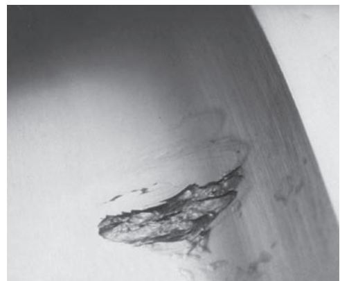
Fig. 5.2 Photo-illustration of fatigue damage on the raceway
